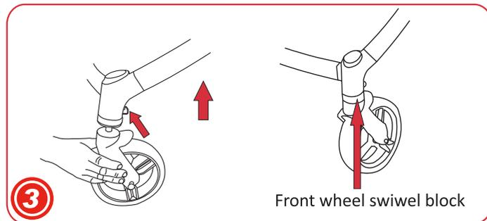
**3 Installing the front wheels**
