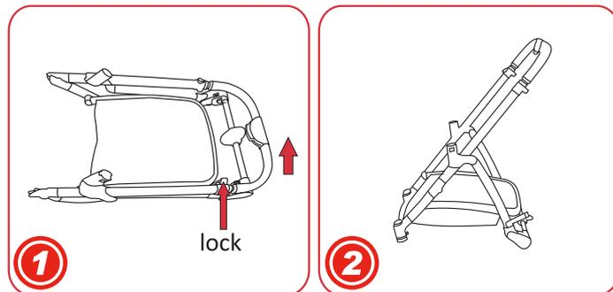
**1-2 Unfolding the stroller**
