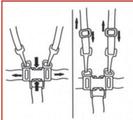
The safety belt has 5 points fastening. Sit down the child in the stroller, fasten seat belts, adjust the shoulder straps in height so that they densely adhered to the shoulders of the child. To unfasten the safety belts, click the button in the middle.
