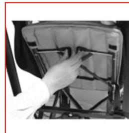
The backrest can be adjusted in 3 positions. Clamp both levers located on the backrest to adjust the tilt, release the lever to fix the backrest in the desired position. To raise the backrest, just push it up.
